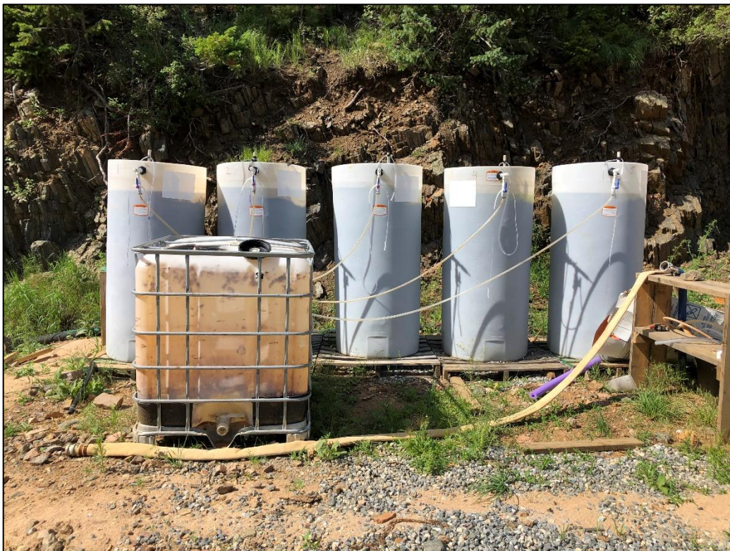
Photo 2. View looking south at BCR system set up for pilot-scale study conducted in area east of water treatment plant.
