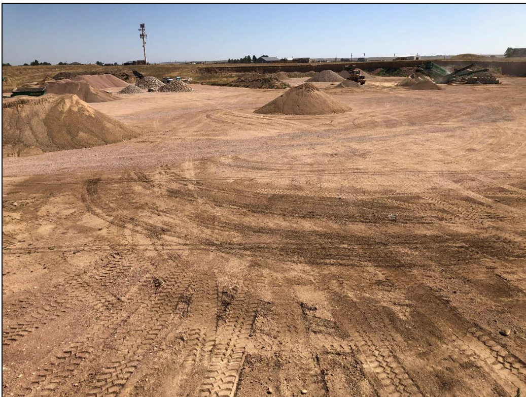
Photo 2. View looking northeast across pit from its southern edge. Note several material stockpiles and portable processing equipment stored on pit floor (in background).
