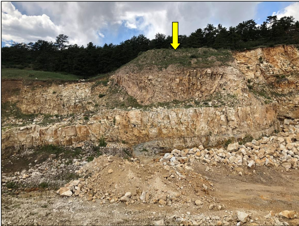
Photo 6. View looking west at western pit wall with mostly 0.5H:1V slopes. Note topsoil stockpile stored above highwall (indicated) stable with vegetative cover.
