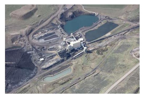
Ponds D and E appears to be holding water and discharging. Construction on stocker coal building appears to be progressing. One tube appears to be up and one ready to install.
