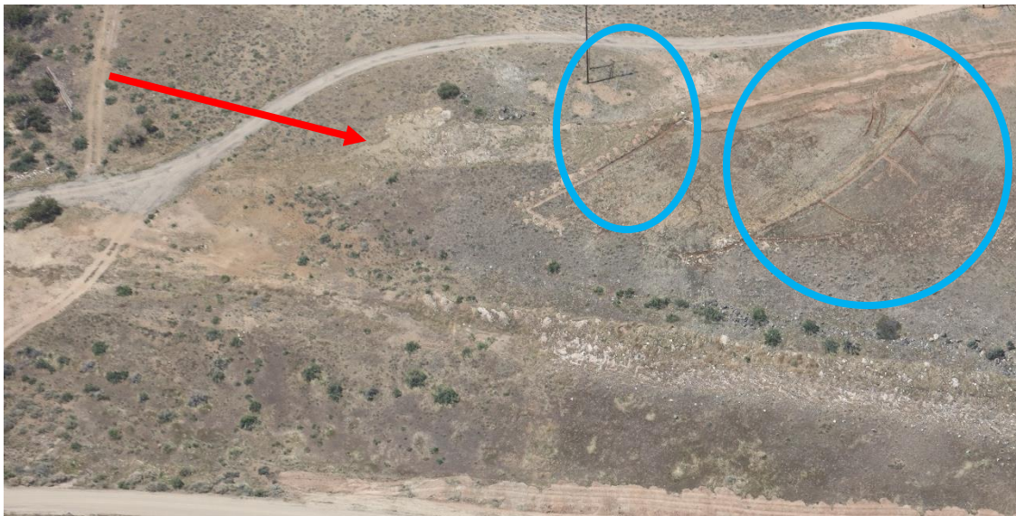
Photo 2: The south end of the Tract 70 Mesa. The blue circles outline the damp locations in the ditches.
