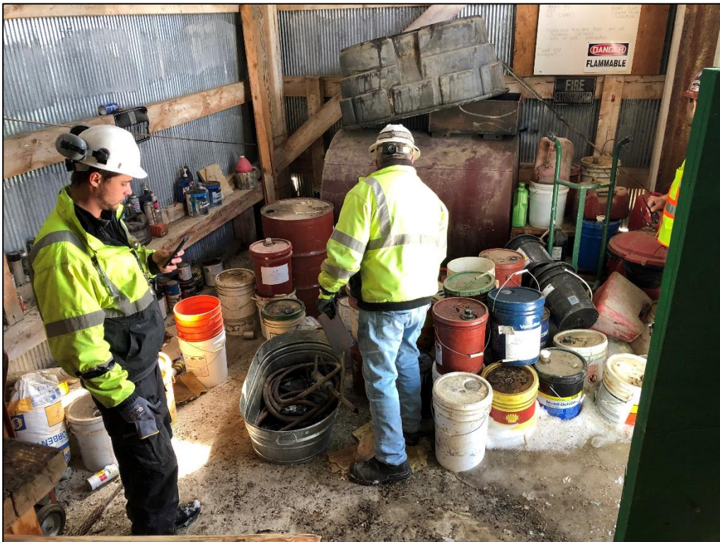
Photo 4. View inside storage shed at Caribou Mine where several containers are stored, most of them empty. This shed should be cleaned up, the containers organized and labeled, and any hazardous materials properly stored.
