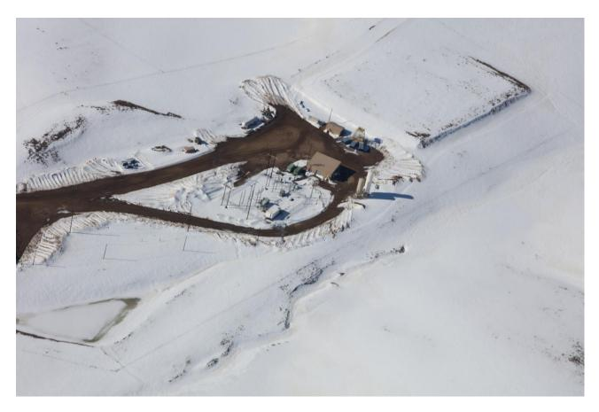
It appears snow removal activities may negatively impact drainage at the site. Shown in the photo above, at the 6MN pad snow appears to have been pushed into the pad perimeter ditch. This will likely impact the proper function of that ditch. Please evaluate snow removal practices and ensure it is not causing off-site impacts. This area will be further evaluated at the next on ground inspection.
