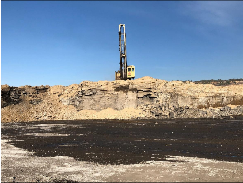
Photo 15. View looking northeast across 3 rd Ridge pit, showing operation drilling along northern pit wall in preparation for blasting.
