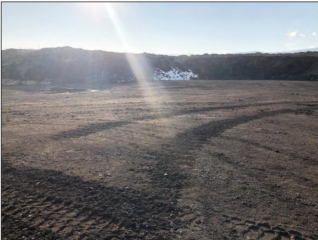
Photo 16. View looking north across 3 rd Ridge pit, showing northern pit wall (in background), approximately 25-30 feet in height with near vertical slopes.
