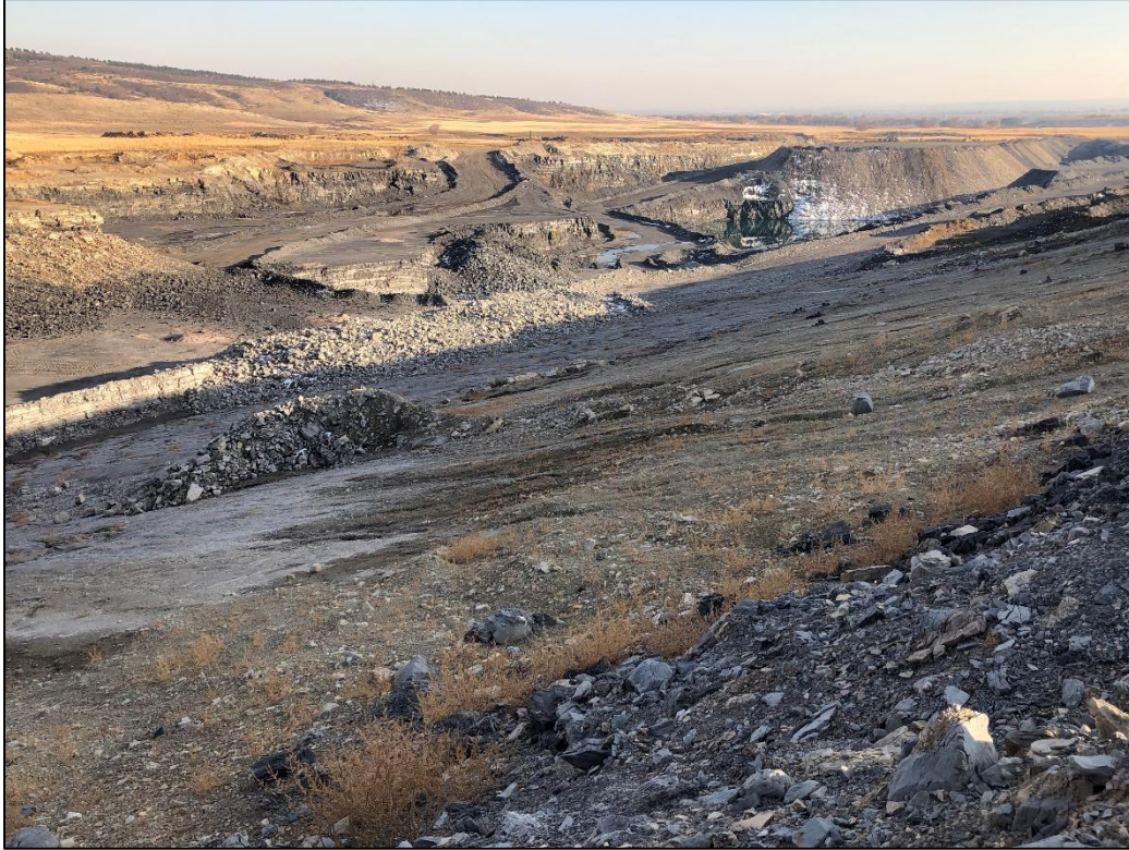
Photo 21. View looking southeast across Hi-Cal pit from its northwestern edge. Note western pit slope (in foreground) graded to 3H:1V or flatter.
