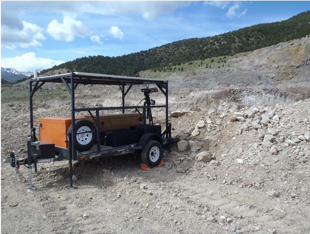
Photo 2. Radar system for monitoring the highwall (NE side of active pit).
