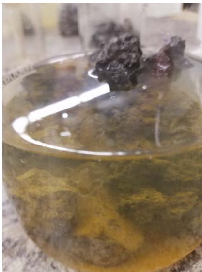
B-Slag when subjected to standing LKA water, after 24 hours.
