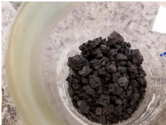
Wet R-Slag material, no obvious signs of precipitation forming on material.
