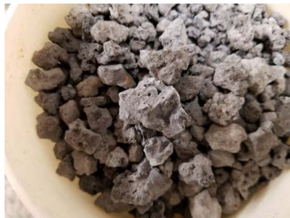
R-Slag material after air drying for 24 hours.
