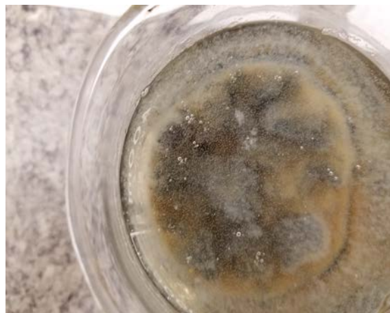
Top view, showing water hardness coming out and forming a salt precipitate on the surface of the water.
