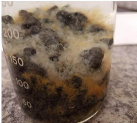
R-Slag when subjected to standing LKA water, after 48 hours.
