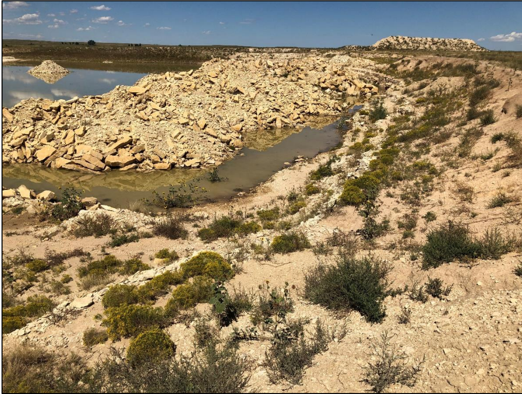
Photo 19. View looking north across eastern pit wall. Note material stockpiled on pit floor. Also note large overburden stockpile at northeastern corner of pit (in background).
