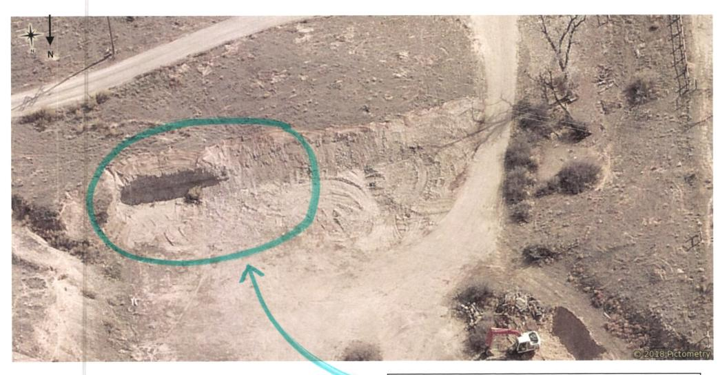
City of Grand Junction GIS Air Photo Date: 03/26/2018 Area of extraction with no contouring to a 3:1 as claimed. Note depth of extraction mined with operator's excavator. Print Date: March 4, 2019
