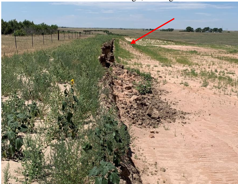
Highwall sloughing on south side of pit looking west. Area where operator has backfilled highwall (red arrow).
