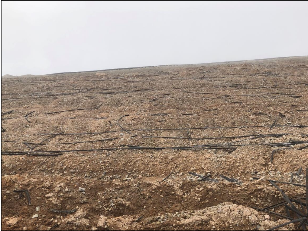
Photo 11. View looking across leaching surface of AGVLF. No solution ponding greater than 3 feet x 3 feet in size was observed.
