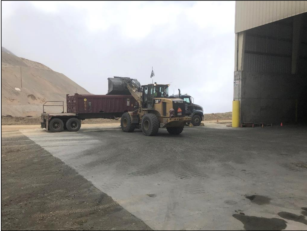
Photo 19. View looking south, showing loader loading concentrate from Con Barn into haul truck during inspection.
