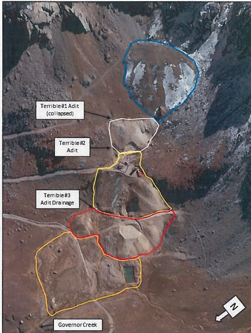
Figure 4. Detailed map of the Virginius and Terrible Mine sites. The Virginius waste rock is outlined in blue. The Terrible #1 mine dump is outlined in white, #2 mine dump in yellow, and #3 mine dump in red. Mixed tailings from the Virginius and Terrible veins are outlined in orange. The polygon boundaries are approximate. Imagery courtesy of Google Earth.
