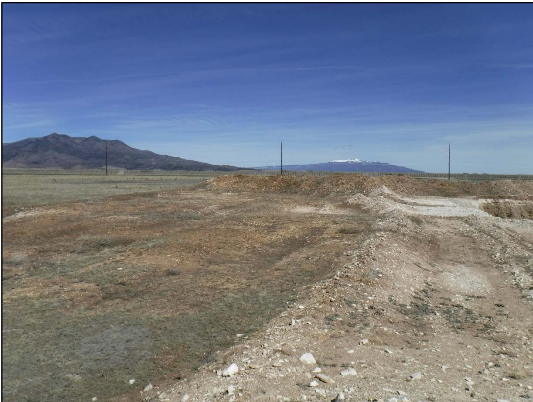
Photo 4: Area stripped of topsoil ahead of mining
