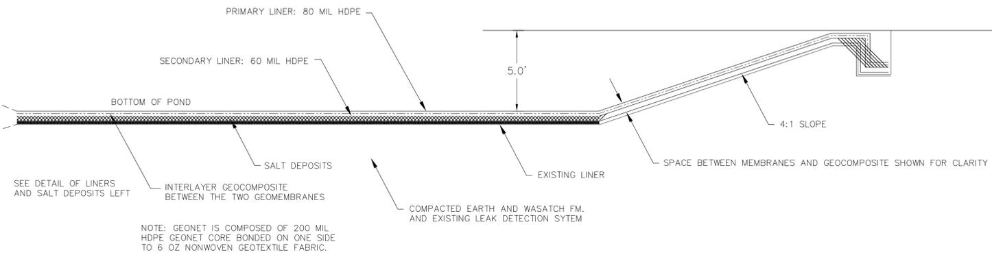
NOTE: GEONET IS COMPOSED OF 200 MIL HDPE GEONET CORE BONDED ON ONE SIDE TO 6 OZ NONWOVEN GEOTEXTILE FABRIC.
