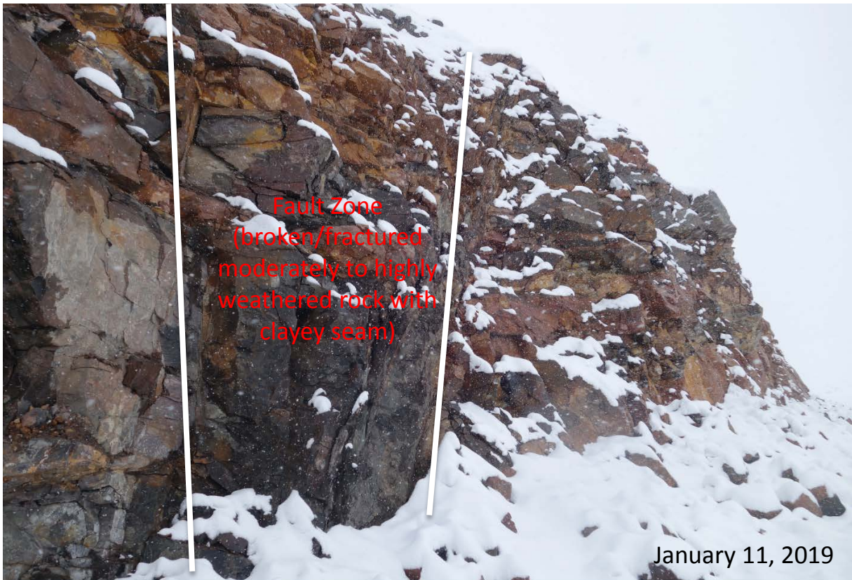
Looking from Station 19-Shear (Figure 2) at near vertical east-west trending fault (3 to 5 feet wide) observed in an actively-mined portion of the Southern Expansion Area at ~EL 6545 ft.
