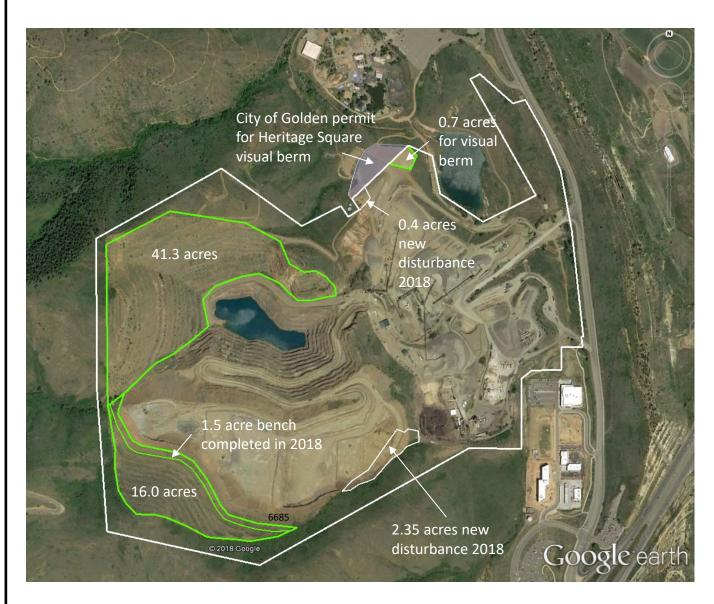
Benches 100% backfilled, graded and seeded
