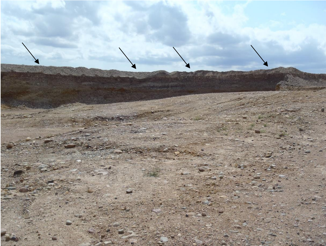
Photo 1. Overburden stockpiled on top of highwalls to construct safety berms (looking SW).
