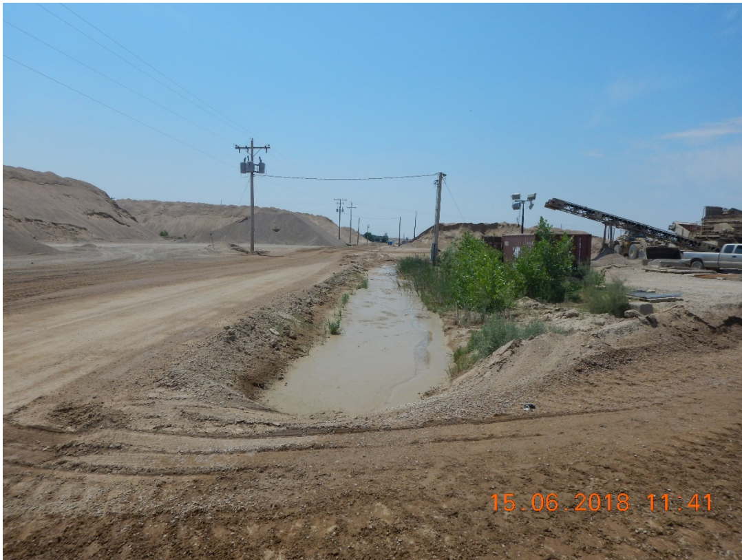
Photograph 3: Control measures not implemented along roadside ditch. Unauthorized process water and stormwater discharge location with a discharge of sediment to the Arkansas River.
