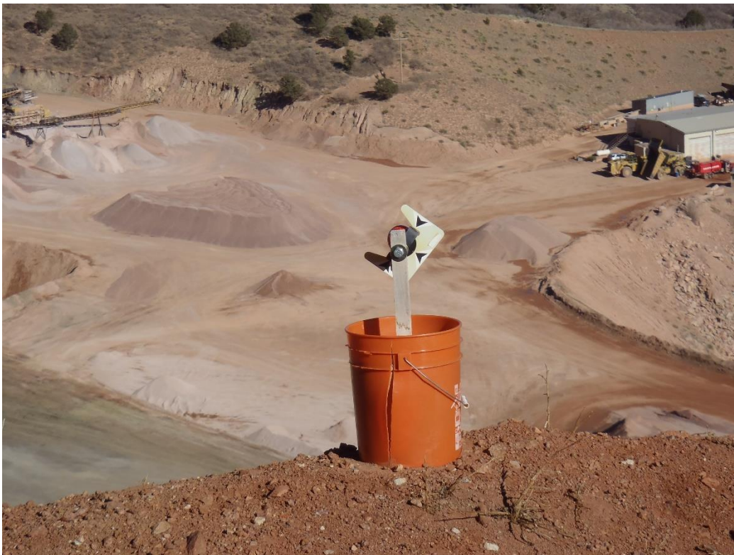
Photo 6. Typical prism for highwall monitoring system.
