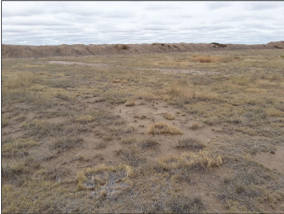
Photo 5. View looking northwest across strip of land located north of active pit where topsoil was stripped in preparation for pit advancement (some years ago judging by the grasses volunteering into the area). The salvaged topsoil is stored along the northern permit boundary (visible in background).
