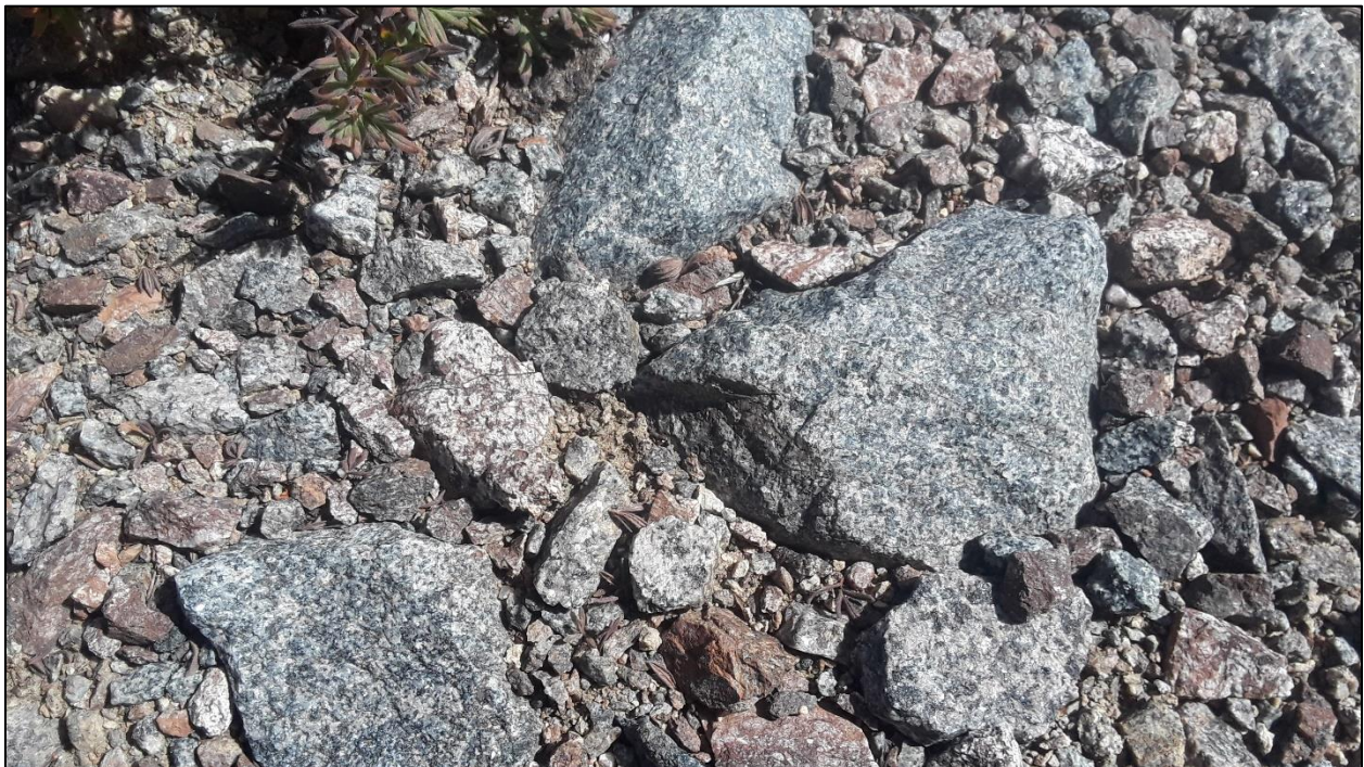
Photo 20. Close-up view of waste rock stockpiled at Caribou Mine, which the operator describes as consisting mainly of quartz monzonite and gneiss.
