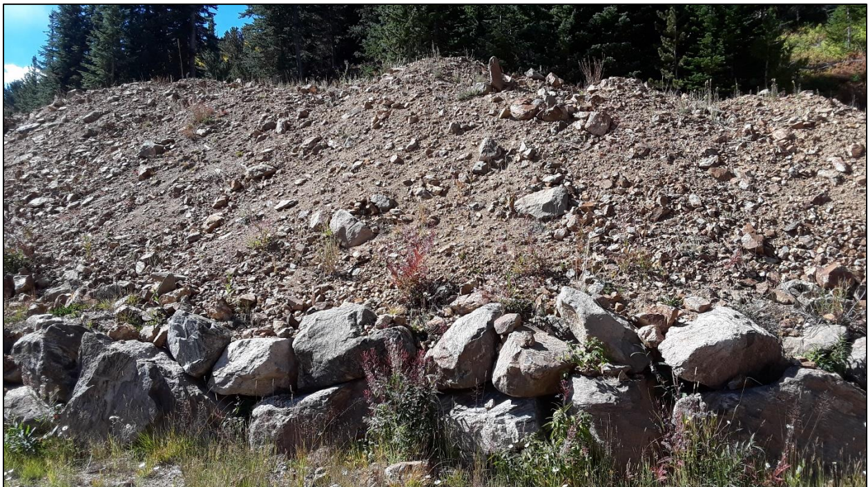
Photo 4. View of waste rock stockpile near Cross Mine Decline portal. Larger rocks were used to construct a retaining wall around the stockpile.
