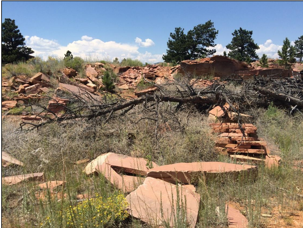
Photo 1. View looking west across south pit area. Large blocks of sandstone scattered across ground will need to be removed from site or used to backfill pits for reclamation. Mine walls will need to be graded to 3H:1V or flatter.
