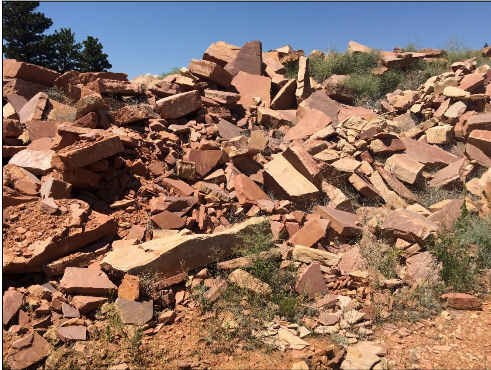
Photo 5. View of rock pile stored in south pit area. This material can be used to backfill the pit for reclamation.
