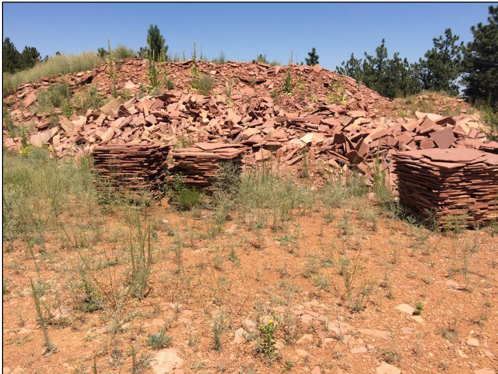
Photo 6. View looking east showing overburden/topsoil stockpile (behind stacked stone) stored at eastern edge of site. This material should be spread across disturbed areas for reclamation.
