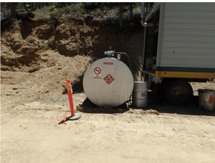
Fuel storage in double wall container
