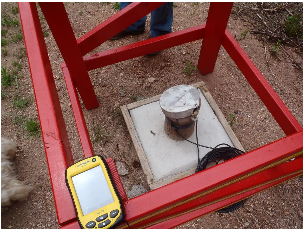
Photo 2. LTC-MW-6 (note unsecured cover and GPS unit).
