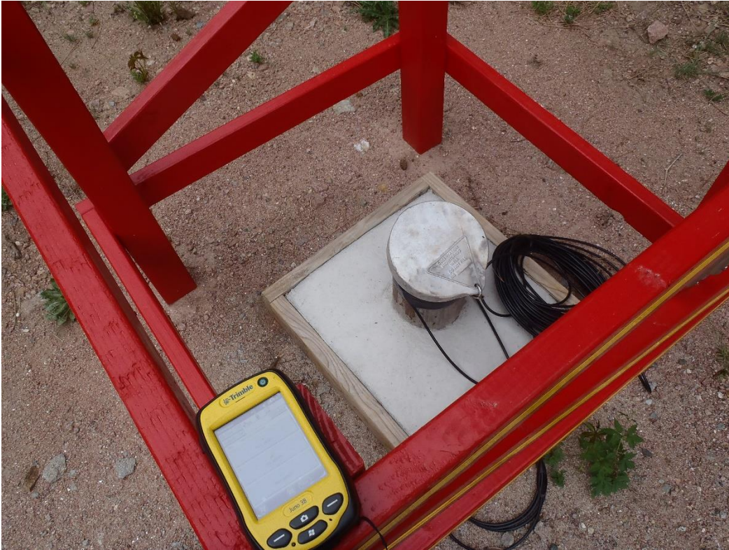
Photo 3. LTC-MW-7 (note unsecured lock on cover and GPS unit).
