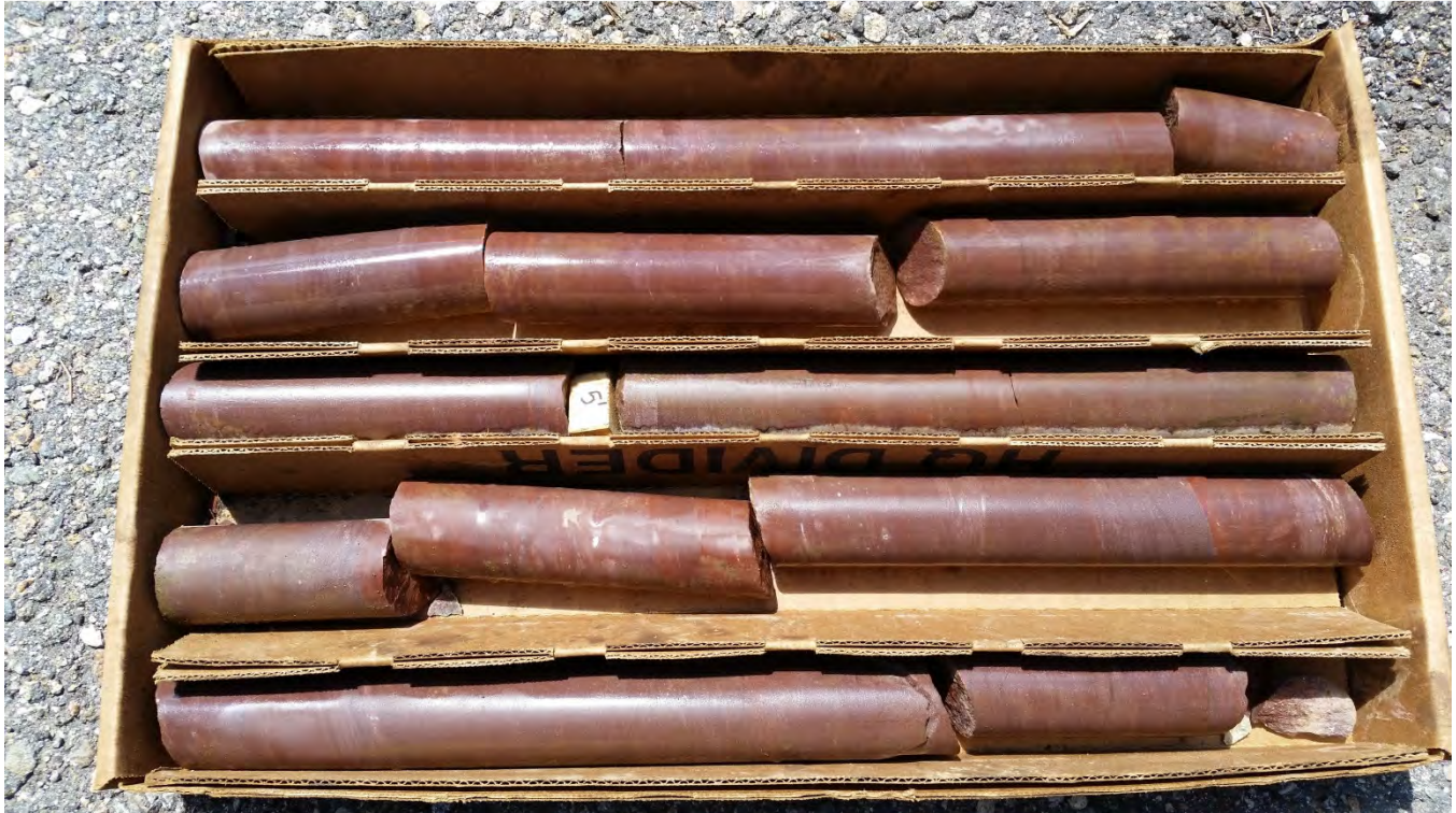
Figure 7: Typical Rock Core (from Borehole U-1 0' to 10' depth)
