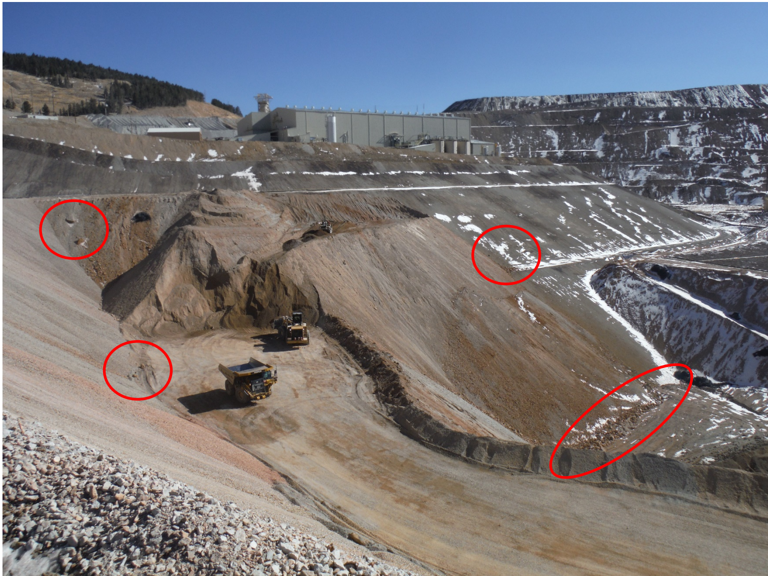
Photos 4. Area of slope failure, non-crushed ore (run-of-mine material) circled in red; looking south.
