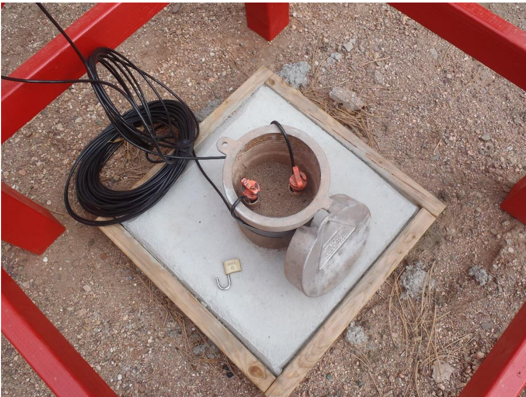
Photo 6. Standard completion (MW-6).
