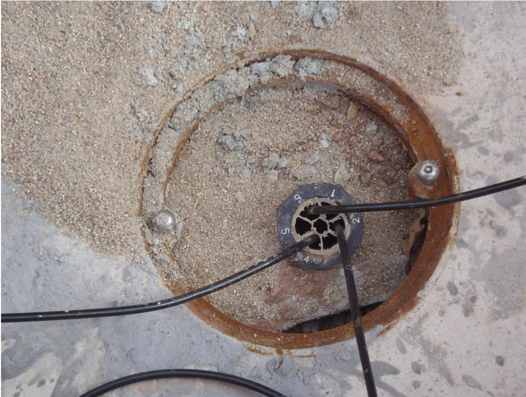
Photo 5. Continuous monitoring well tubing (MW-7).
