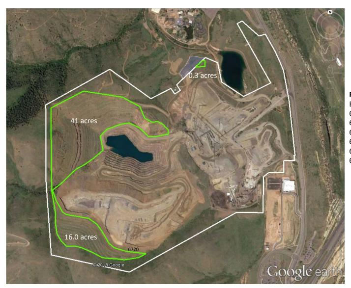
Benches 100% backfilled, graded and seeded
