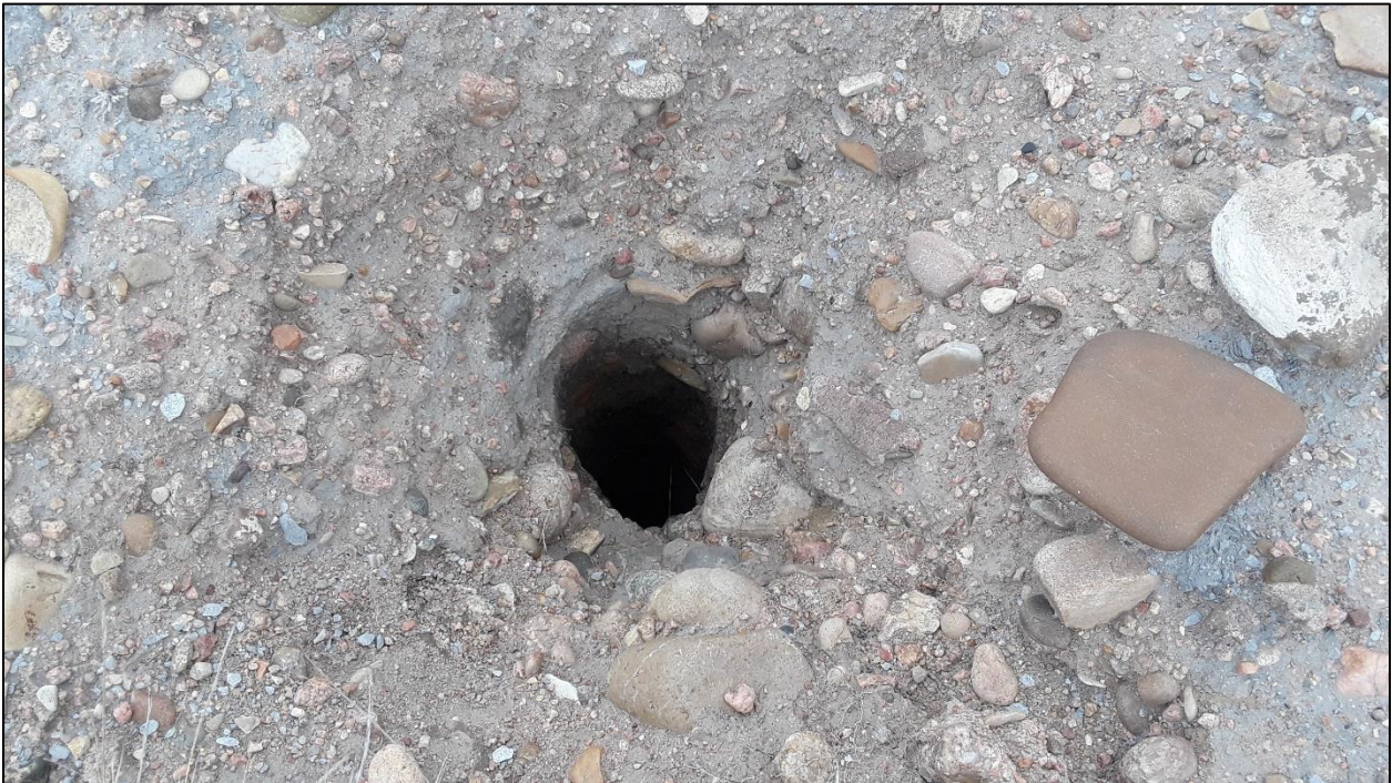
Photo 6. Close-up view of borehole DH3 located near center of M-2013-008 permit area. Borehole was approximately 4 feet deep and dry.
