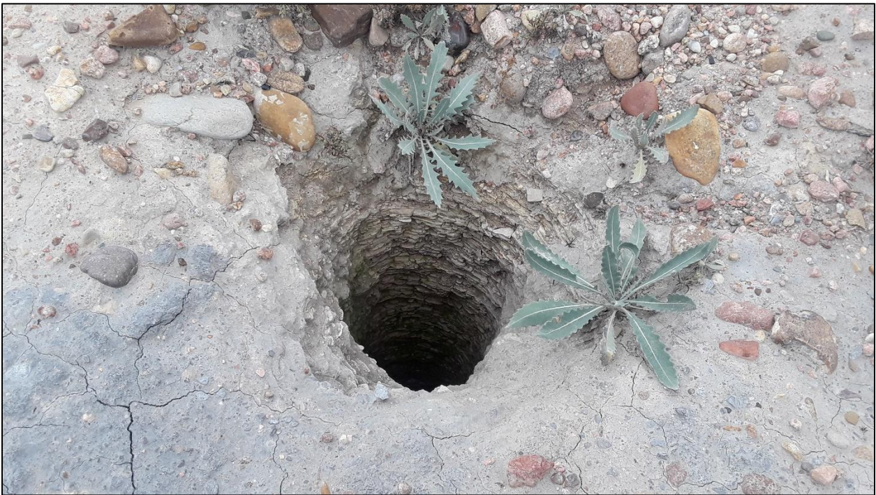
Photo 4. Close-up view of borehole DH1 located at southern edge of M-2013-008 permit area. Borehole was approximately 8 feet deep and dry.
