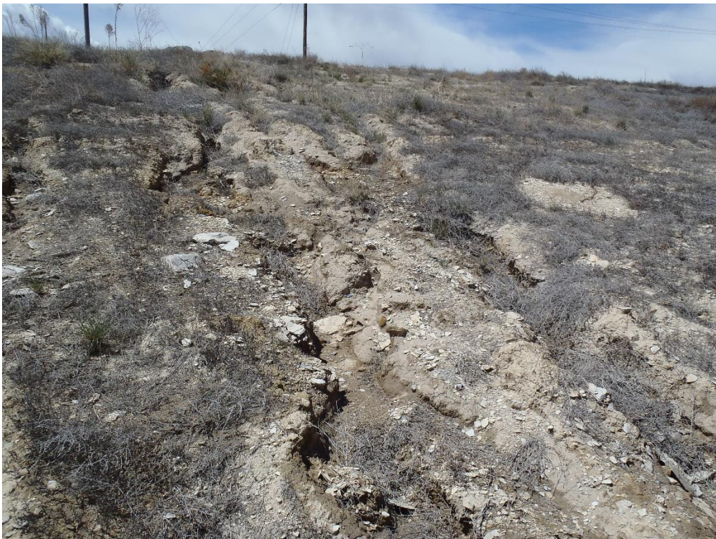
Photo 6. Erosion rilling and gulying observed along the Bear Creek realignment.
