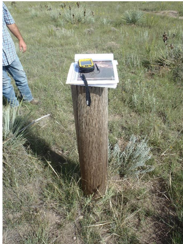
Photo 3. Trimble Juno 3B used to collect position of each permit boundary corner marker.
