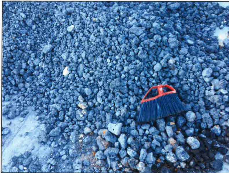
Photo 2. Slag material after processing on site by Golden Wonder staff and screened through 5/8-inch screen. Photo was taken looking into a bag of processed slag.
