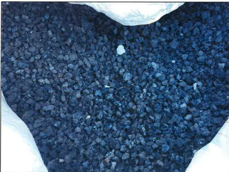
Photo 2. Slag material after processing on site by Golden Wonder staff and screened through 5/8-inch screen. Photo was taken looking into a bag of processed slag.
