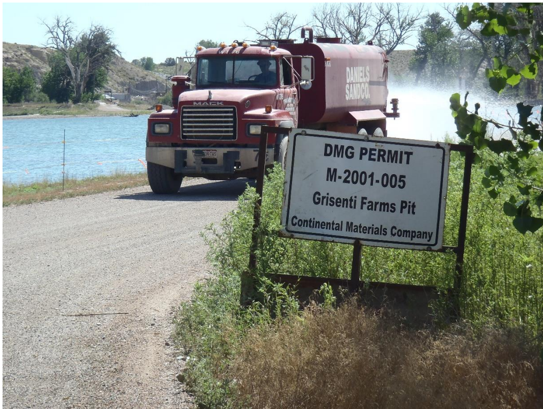
Photo 1. Posted permit sign and active dust control using water truck.
