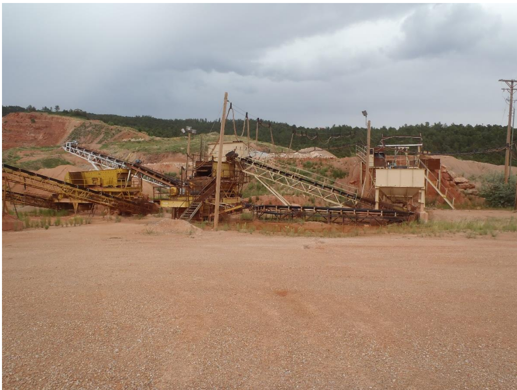
Photo 6. Screen plant, conveyor, and crusher (south pit, looking SE).
