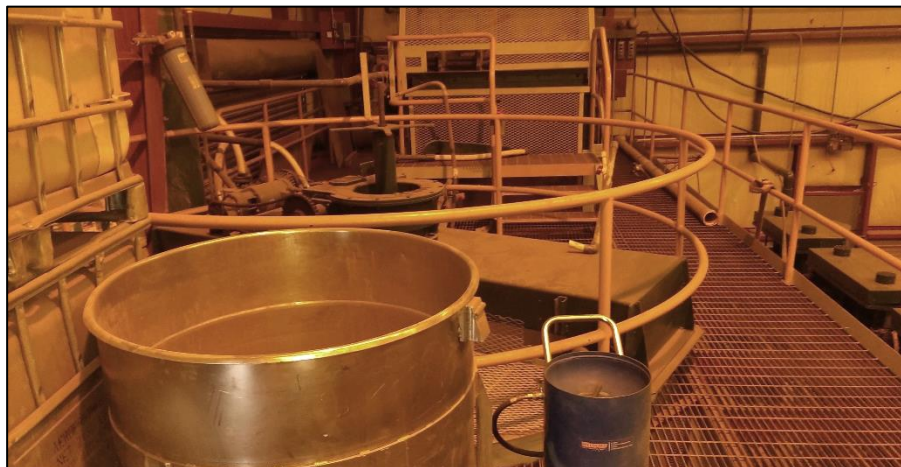
Photo 21. View inside mill showing deck where concentrated pump enters a disc vacuum filter (in background) to dewater the concentrate in preparation for shipment.
