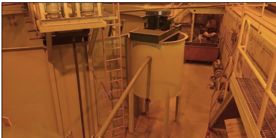
Photo 18. View inside mill showing conditioner tank (adjacent to thickener tank) where reagents are added to pulp before entering flotation circuit. Most likely, reagents will include a readily soluble frothing oil (i.e., pine oil, cresol) and quick-acting promoting reagent (i.e., xanthate).
