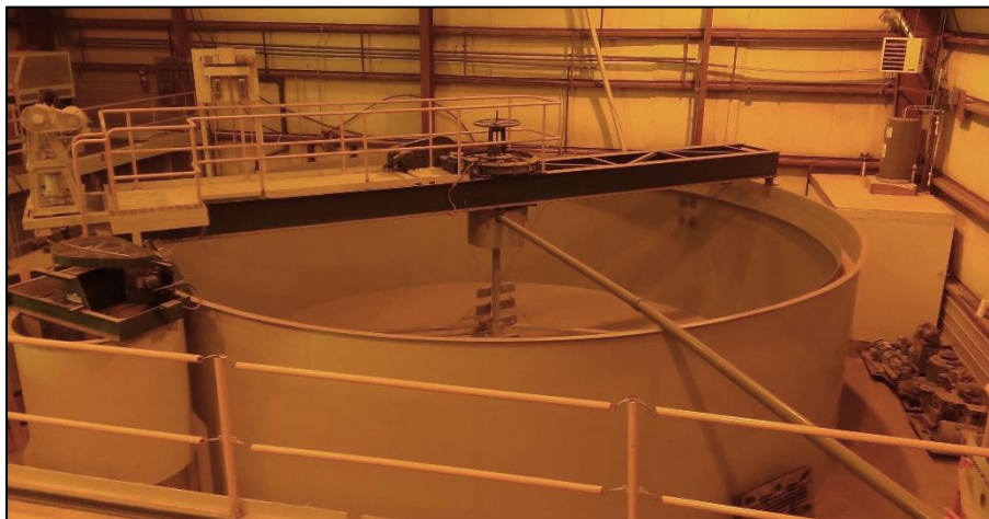
Photo 17. View inside mill showing large thickener tank where overflow from shaking table carries suspended, finely divided fraction of pulverized ore. This tank clarifies mill water which is returned to ball mill for recycling, and increases concentration of suspended solids prior to flotation.
