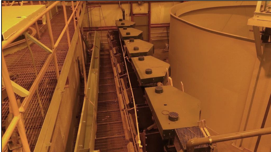
Photo 19. View inside mill showing flotation circuit composed of 8 cells where conditioned pulp enters for final concentration. Final concentrate pulp is collected for filtration, while tailings are pumped to tailings impoundment.
