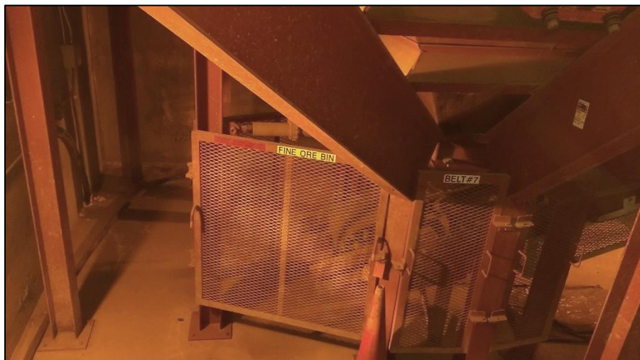
Photo 15. View inside mill showing fine ore bin where crushed ore is stored until conveyed to grinding circuit to complete comminution process.
