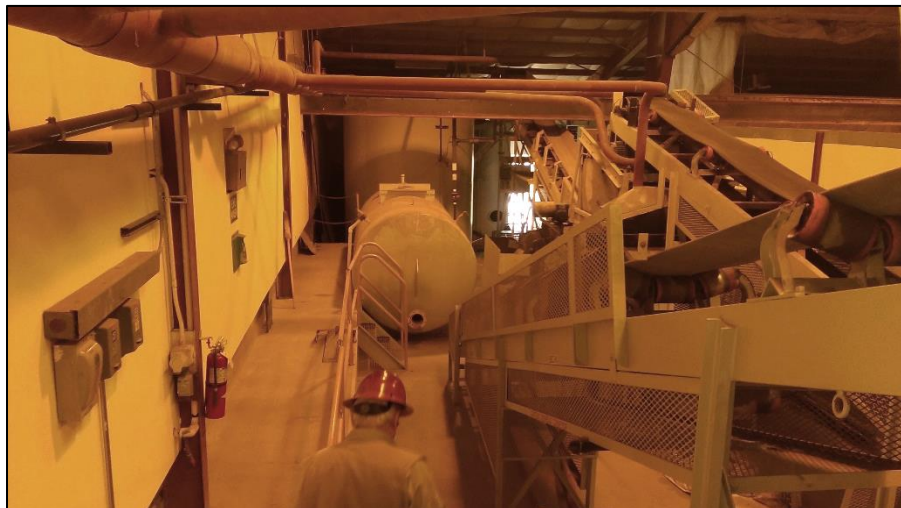
Photo 14. View inside mill showing closed-circuit crushing plant. No water is added in this circuit. A dust-collection system is in place (including red pipeline shown at top of photo).
