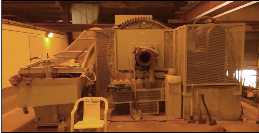
Photo 16. View inside mill showing closed-circuit grinding plant, which includes a ball mill and a spiral classifier. Fresh water is added to ore at this phase for wet grinding. Soda ash is added to control pH levels.
