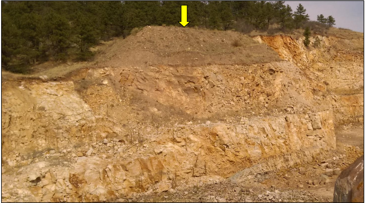
Photo 9. View looking west from southeastern edge of pit, showing topsoil stockpile stored at top of highwall (indicated with arrow).
