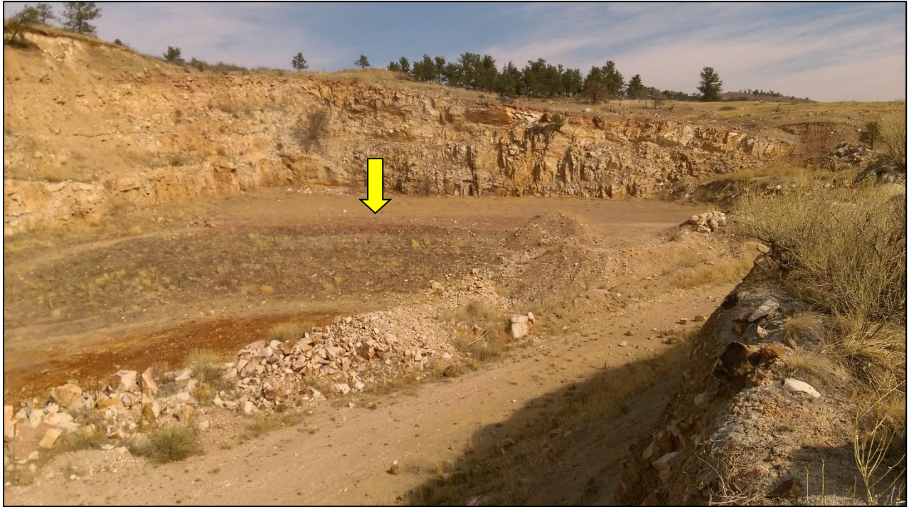
Photo 5. View looking north from eastern edge of pit, showing northern highwall (in distance). Note portion of pit floor (indicated with arrow) that was backfilled and seeded in 2014.
