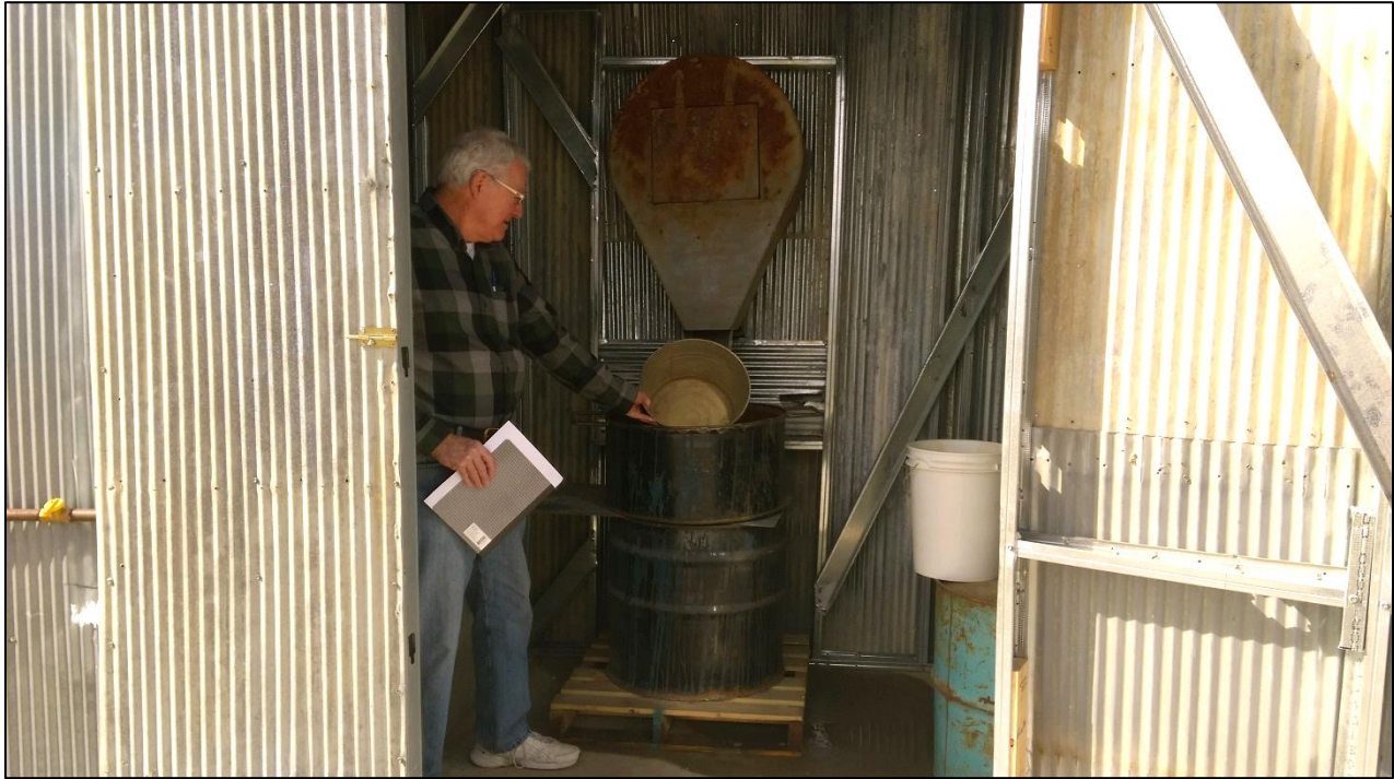
Photo 5. View of output end of roaster where material would come through at approximately 5 gallons per load.
