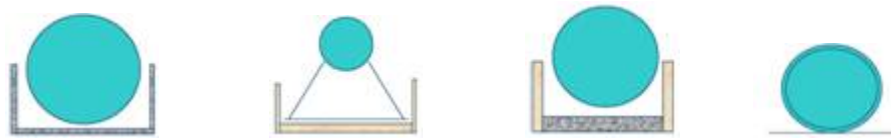
Examples of Category 1 ASTs with adequately sized and impermeable secondary containment. (e.g. spill control and release prevention barrier (RPB))
