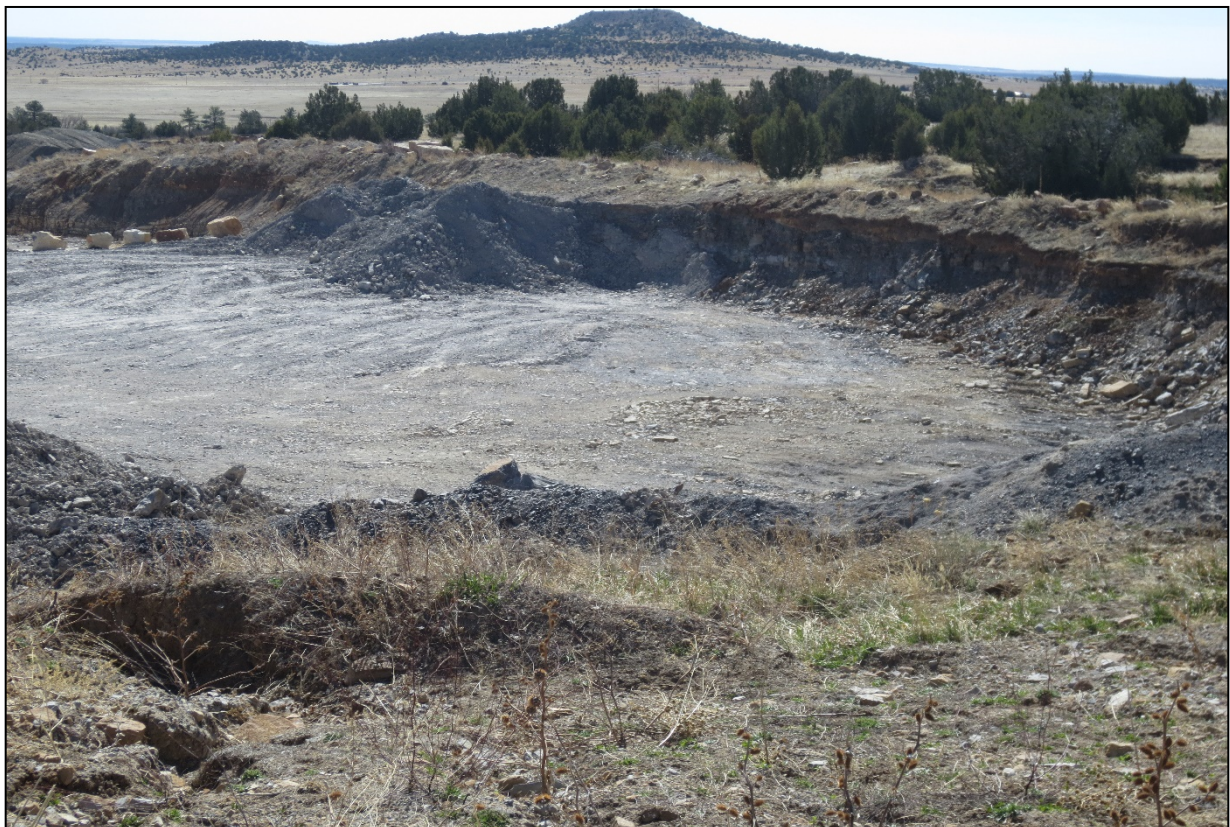
Photo 1: Recent mining operations, sandstone has been mined off exposing the clay.
