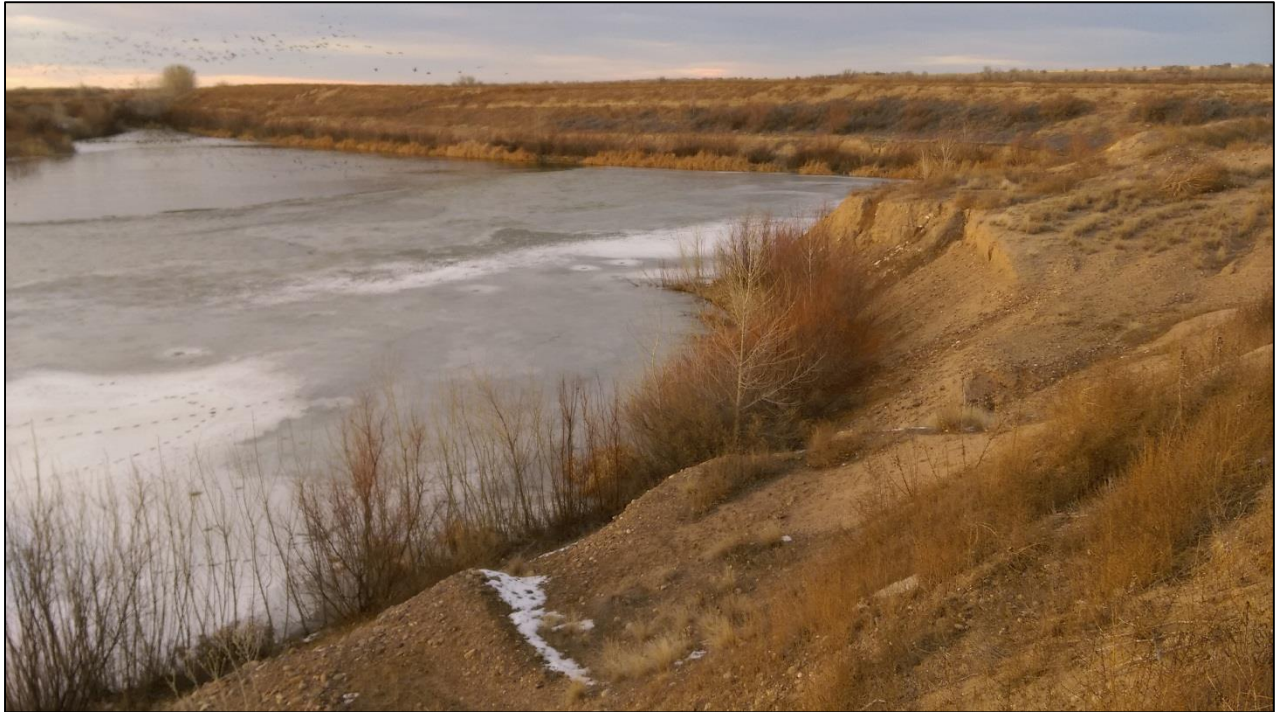
Photo 10. View looking north, showing smaller pond (4.1 acres in size) located in east mining area (eastern shoreline shown in foreground). Note shoreline slope gradients steeper than 3H:1V.
