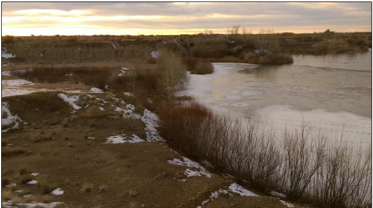
Photo 12. View looking southwest, showing smaller pond (4.1 acres in size) located in east mining area (eastern shoreline shown in foreground). Note shoreline slope gradients steeper than 3H:1V.
