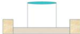
Example of a Category 2 ASTs with an adequately sized earthen berm but no CDRM.
