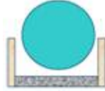
Examples of Category 1 ASTs with adequately sized and impermeable secondary containment. (e.g. spill control and release prevention barrier (RPB))
