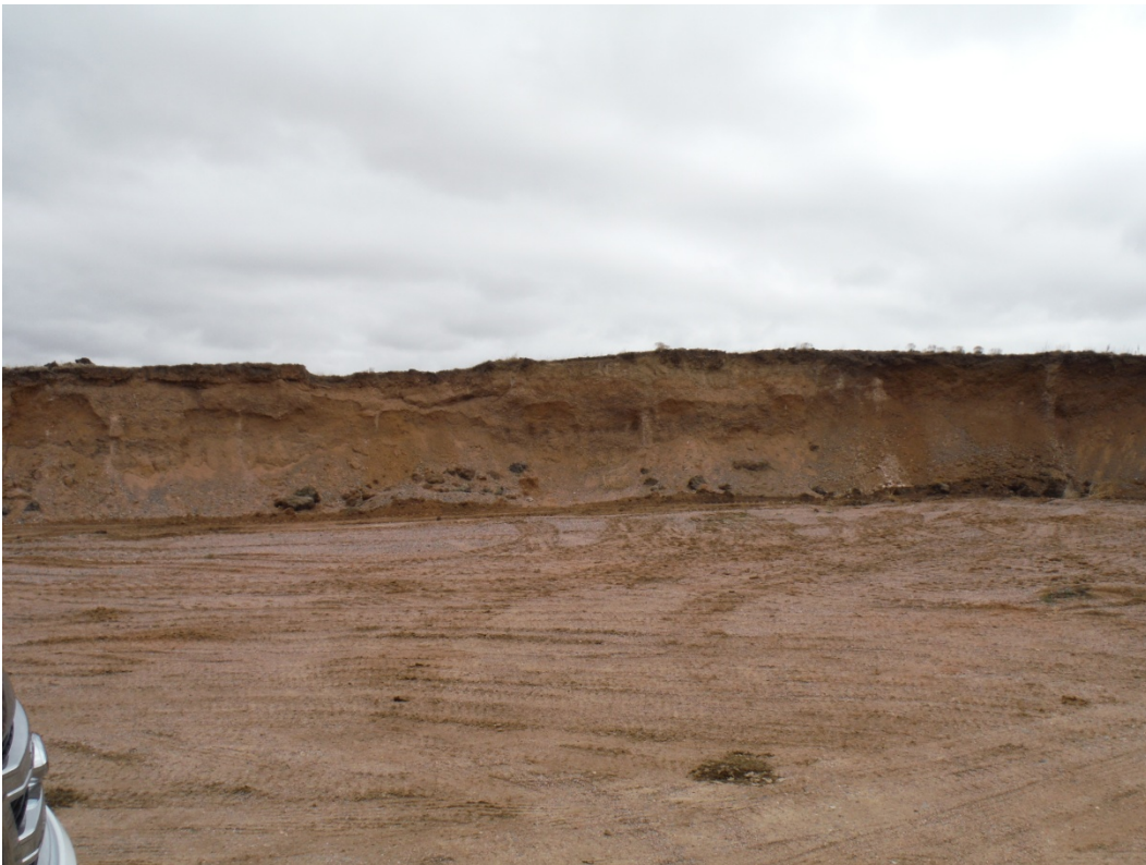
Pit active mining face (note: darker organic “topsoil” sloughing off due to not being stripped); looking south.
