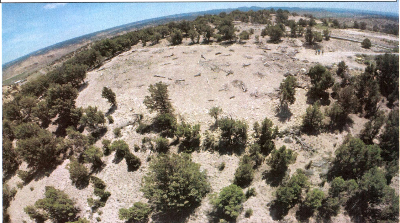
Photo 13 – Production well pad 20-30 after re-contouring and drill seeding. Photo taken June 2015. Reclamation work is completed in late fall to allow for overwinter seeding which enhances germination.
