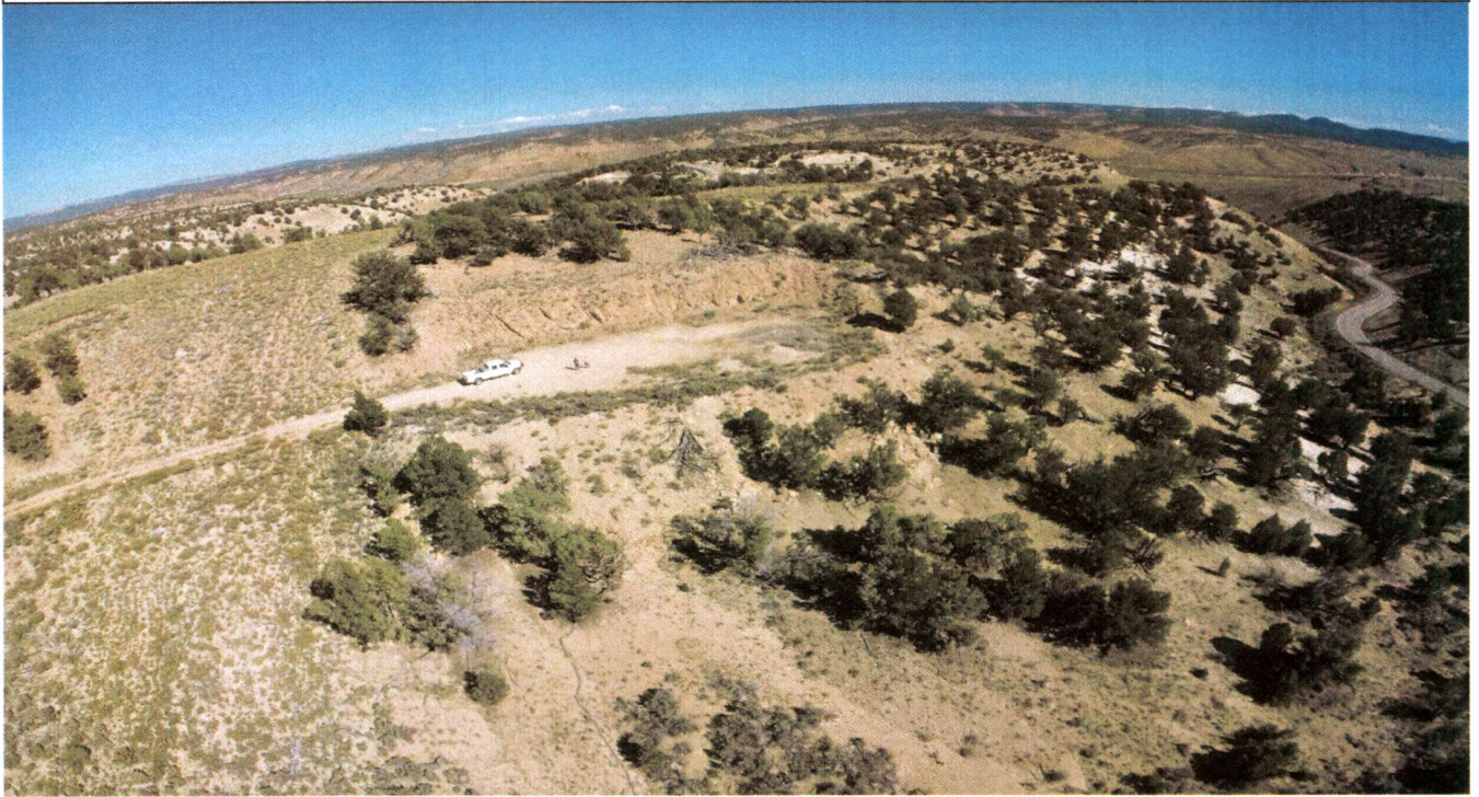
Photo 6 – Production well pad 20-35 was plugged and abandoned in September 2004. In the fall of 2014 the piping and well skid were removed and the well pad re-contoured and reclaimed. A reclaimed natural gas pipeline corridor can be seen on the left side of this photo taken in fall 2014.
