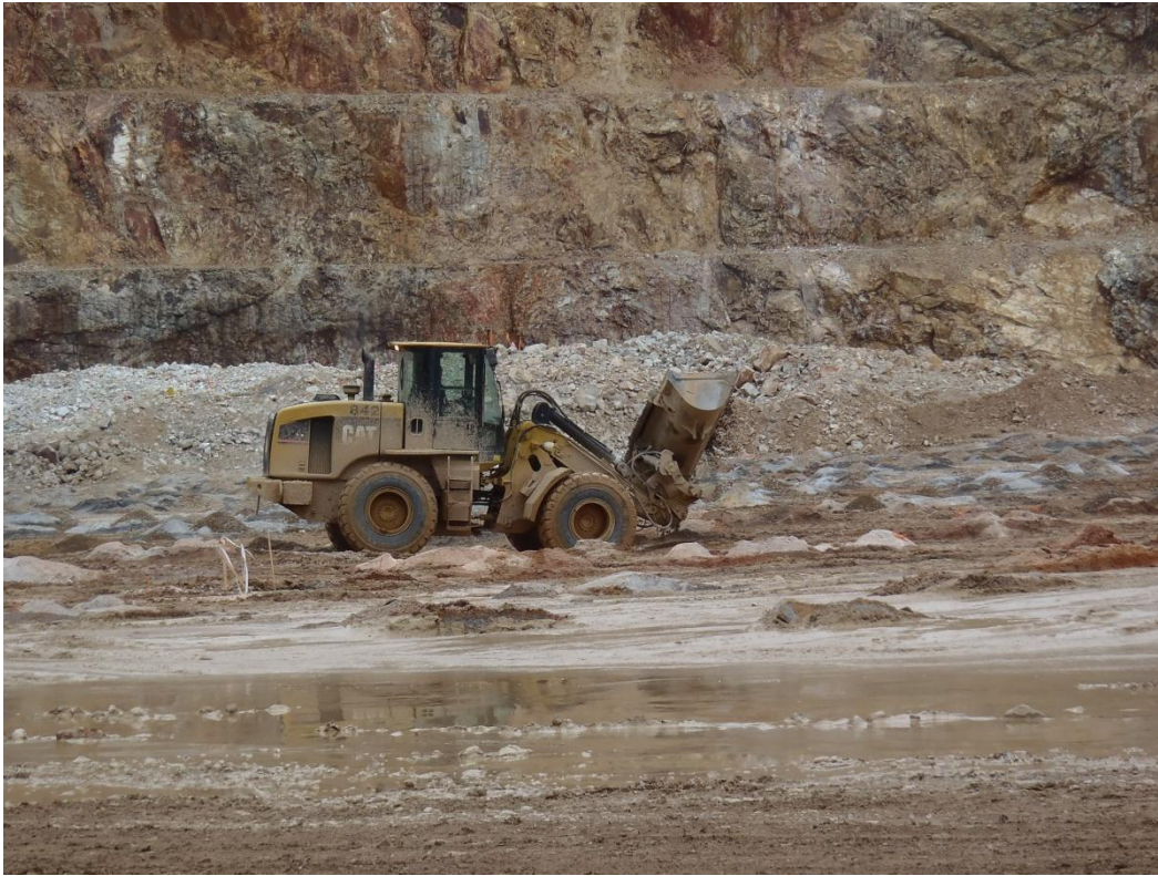
Photo 1. Side tipping loader filling blast holes with stemming material (WHEX Pit).
