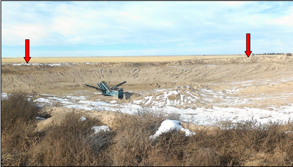
Photo 3. View looking north into mined pit from top of southern pit wall. Note mined slopes kept at 3H:1V gradient or flatter, and topsoil stockpiled in berms around edges of pit (indicated).
