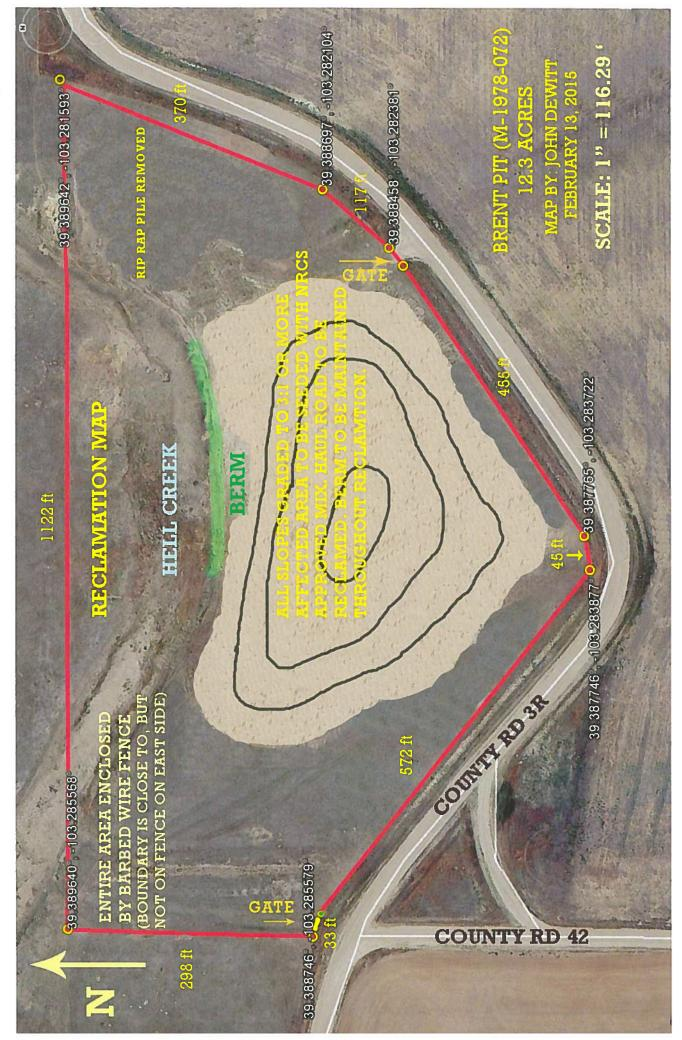
39 388697 -103 282104 SCALE: 1'' = 116.2939 389642 -103 281593 39 388458 , -103 282381 REINT PIT (M-19) STOCK PILE **39** 387765 -103 283722 AREA HELL CREEK 1122 ft LION 39 387746 -103 283877 COUNTY ROSE NOT ON FENCE ON EAST SIDE) (BOUNDARY IS CLOSE TO, BU BY BARBED WIRE FENCE ENTIRE AREA ENCLOSEI 39 389640 -103 285568 39 388746 -103 285579 GATE COUNTY RD 42
